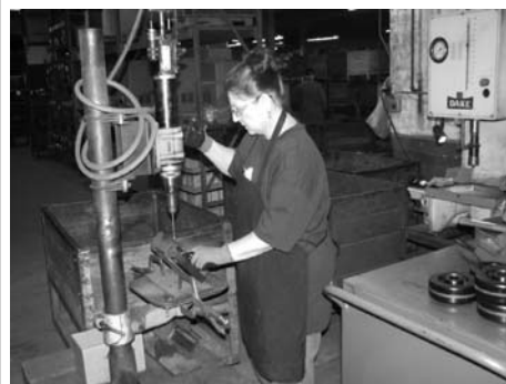
Old trigger controls (shoulder level)
