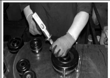
New hammering station (wheel stabilized)
