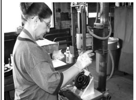
New triggering controls (below chest level)
