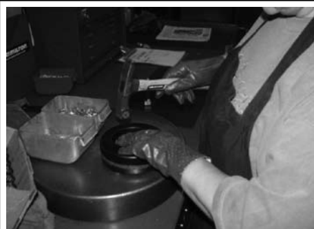
Old hammering station (wheel not stabilized)
