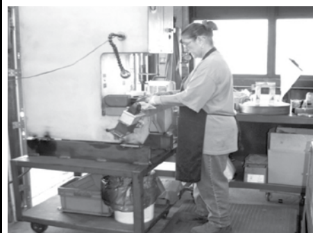
Modified hydraulic press (raised 4")
